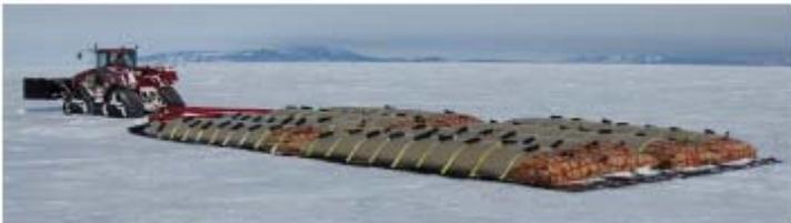
Figure 3 Traverse tractors towing eight fuel bladders.
