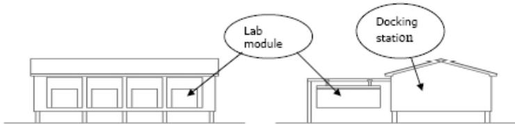
Figure illustrating docking station with containerized laboratories.
