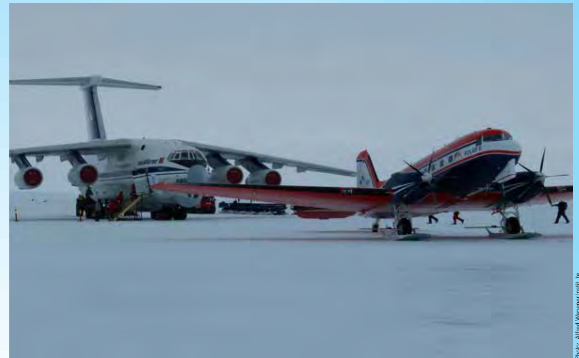
The Ilyushin 76 (IL-76) and Basler 67 (BT-67) aircraft at ice runway in the Dronning Maud Land area
