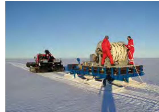
Vibroseis traverse showing snow streamer being deployed on the Ekström Ice Shelf
