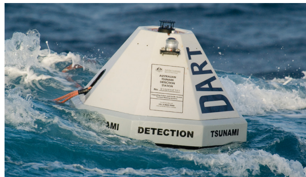
A Deep-ocean Assessment and Reporting of Tsunamis (DART) buoy
