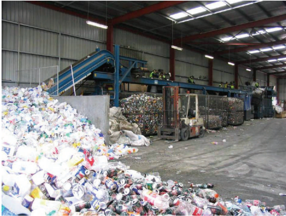
Figure 2: Recyclables can be received co- mingled from Antarctica for sorting in the Collex / Veolia recycling facility in Hobart
