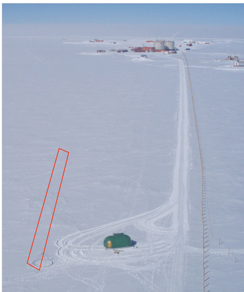
Figure 2- Area over which BRDF measurements were taken (inside red box). Measurements were taken at 8 sites spaced at ~10m intervals, each site further towards the base.
